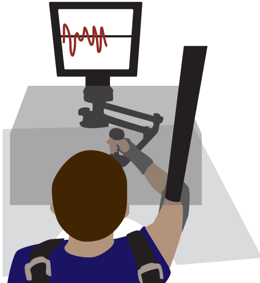
Figure 4-8: Experimental setup. The InMotion2 simulated a virtual circular constraint. Vision of the arm and robot were occluded. The subject was provided with visual speed feedback. The wrist was braced, the elbow was supported by a sling, and the shoulders were strapped to a chair.
